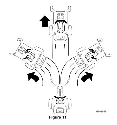
To turn, pull back on the motion control lever toward the direction you want to turn (Figure 10 and Figure 11).
